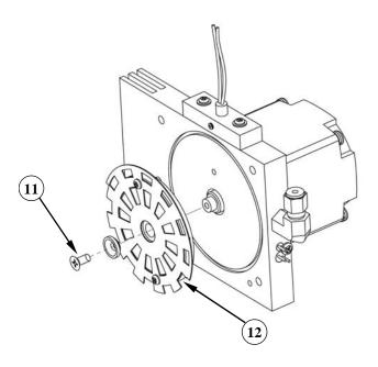
Figure 12-18: Removing the GFC Wheel
